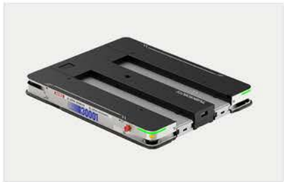
TUSKE Compatible with National and European Standard Pallets. Lifts up to 800kg. Stop accuracy: ±5mm/±1°.
